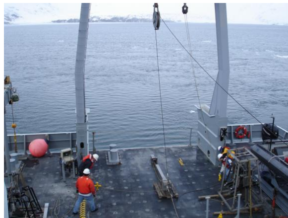
Figure 5: Picture of Kasten core being recovered on the stern of the R/V Thompson in North Tarr Inlet(photo by Eric Collins).
