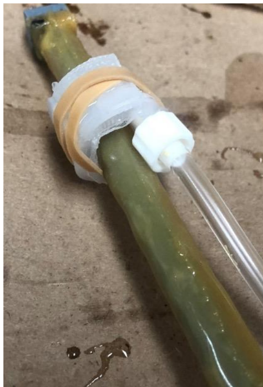
Figure C1: Urethra Core mold + Sphincter Device combination to create prostatic sphincter.
