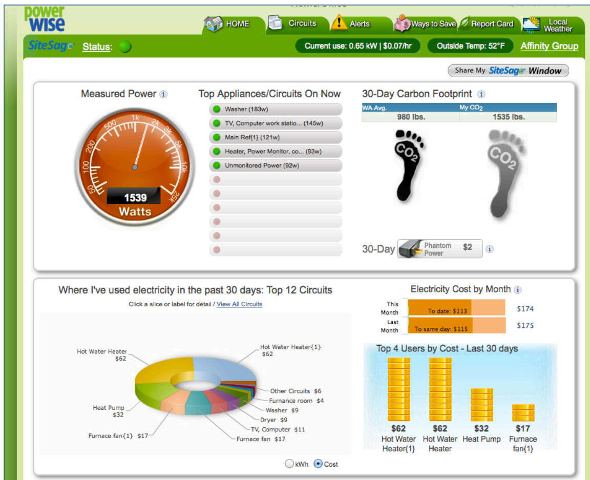
Figure 3.12. Example of PowerWise / SiteSage Dashboard.
