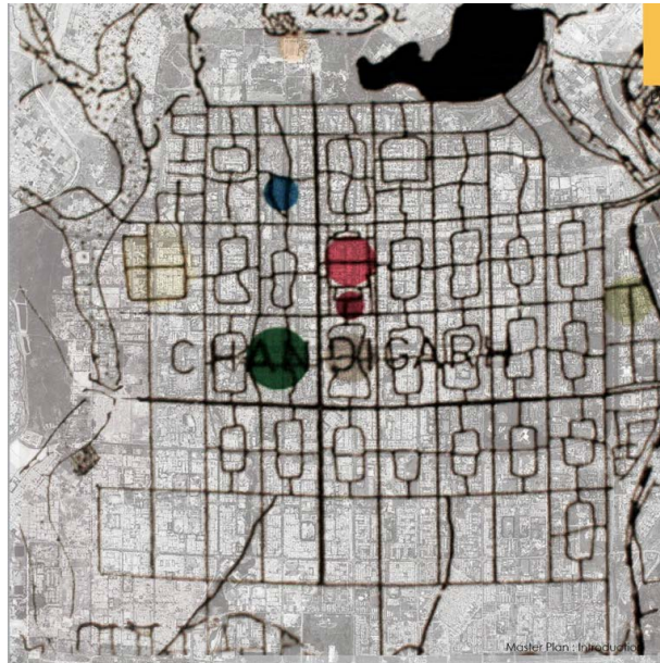
Figure 3.11 - Overlays of Le Corbusier's master plan diagram and satellite image of Chandigarh in 2010 Source Chandigarh Urban lab
