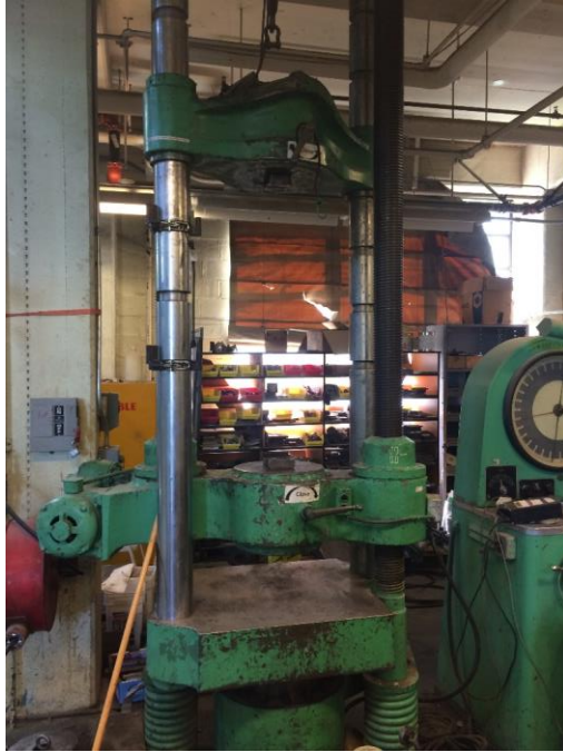
Figure C-3: 300 Kip Baldwin testing Machine
