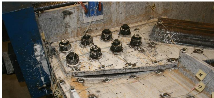
b. Moderate local buckling (PS LB2, 2.3%)
