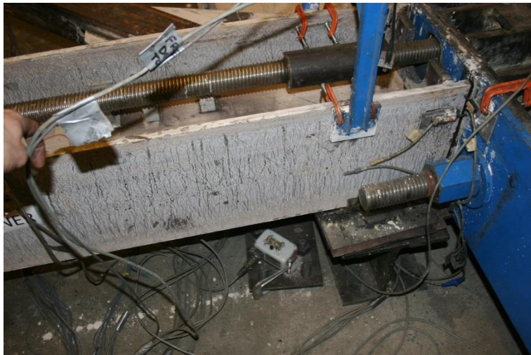
Figure 5-72: Initial Yielding in W Column Outer Flange (PS Y1-OF, 3.7%)
