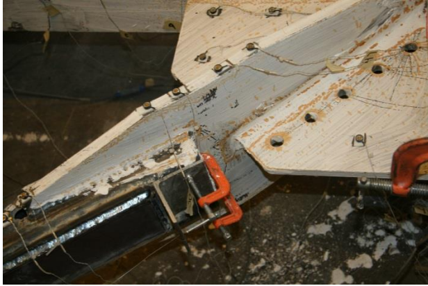
a. Tension Side of Knife Plate
