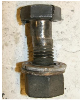
b. Bolt Shear Deformation
