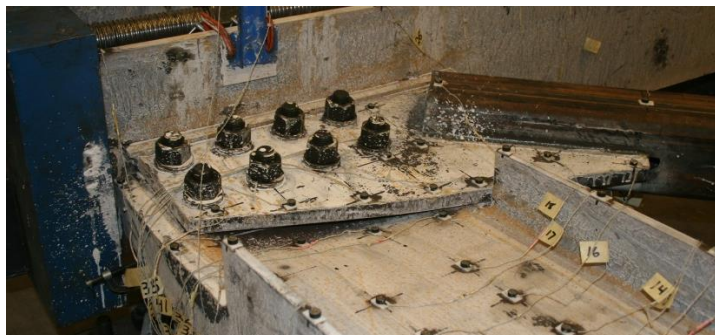
c. Severe Local Buckling (PS LB3, 2.2%)
