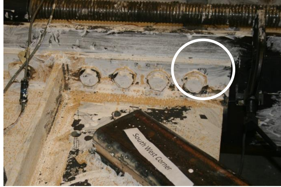
Figure 5-13: Initial Yielding in SW End Plate (PS Y1, 1.6%)
