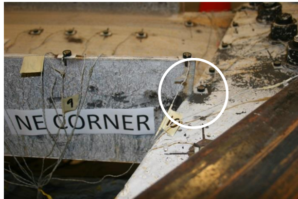
Figure 5-70: Local Yielding from Beam-to-Gusset Plate Contact (3.7%)
