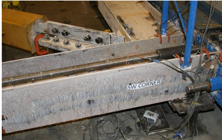
Figure 5-88: Initial Yielding in W Column Outer Flange (PS Y1-OF, 3.4%)
