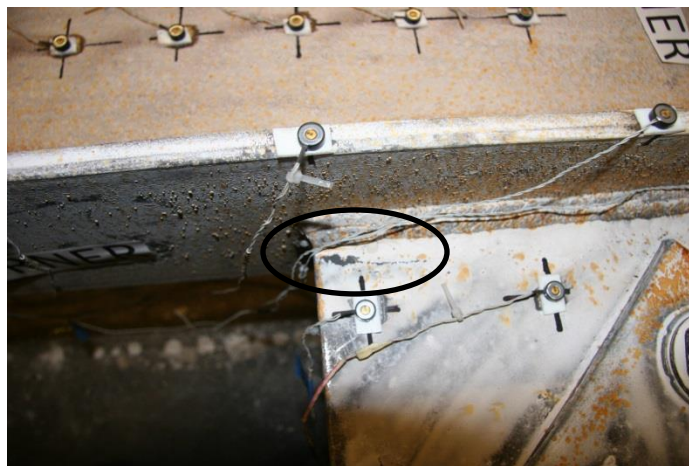
Figure 5-84: Initial Yielding in the NE Gusset Plate (PS Y1, 1.0%)
