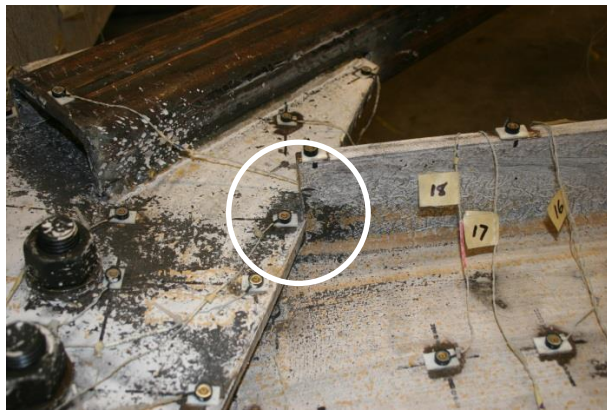
Figure 5-70: Local Yielding from Beam-to-Gusset Plate Contact (3.7%)
