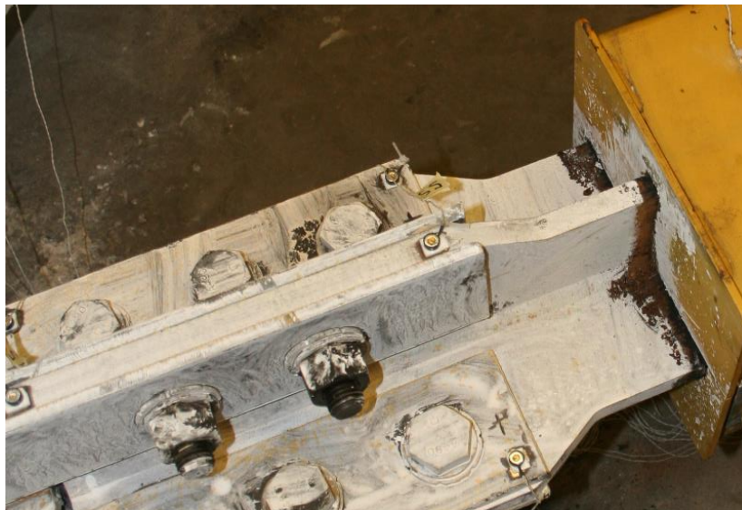
Figure 5-48: BRB Core Plate Moderate Yielding (PS B2, 2.0%)
