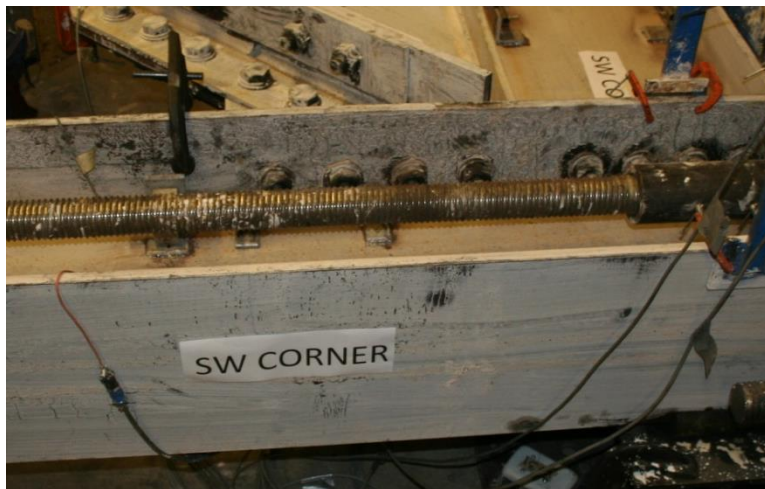
Figure 5-52: Initial Yielding in the West Column Outer Flange (PS Y1-OF, 3.0%)
