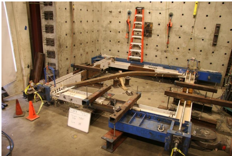
Figure 5-68: Moderate Brace Global Buckling (PS B2, 2.7%)
