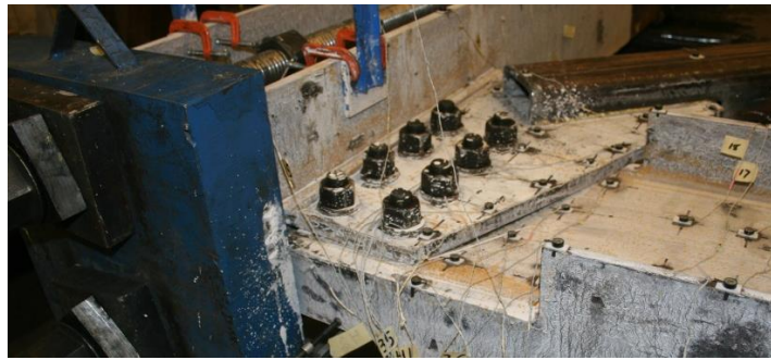
a. Initial Web Local Buckling (PS LB1, 1.9%)
