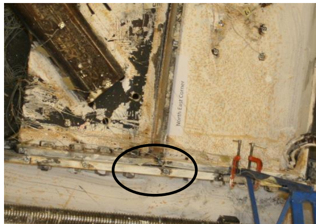
Figure 5-17: Prying Action of NE End Plate (PS P2, 2.9%)
