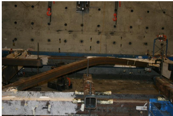
Figure 5-14: Moderate Brace Global Buckling (PS B2, 2.3%)
