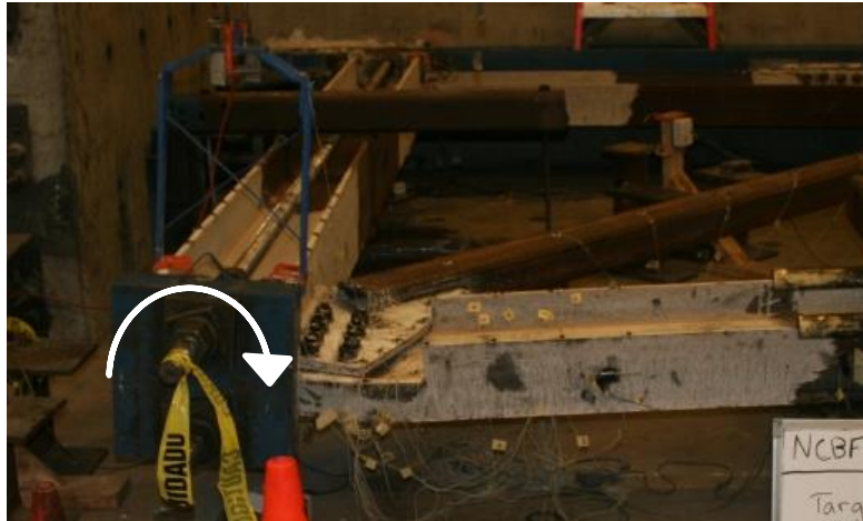
Figure 5-65: Twisting of E Column (2.7%)
