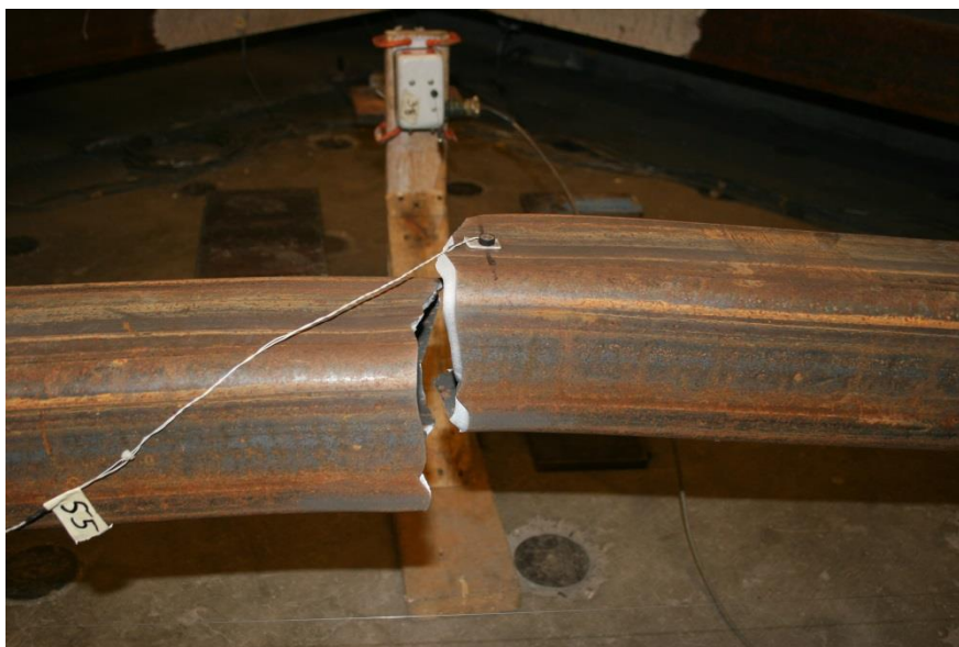
Figure 5-75: Brace Fracture (PS B4-BF, 5.0%)
