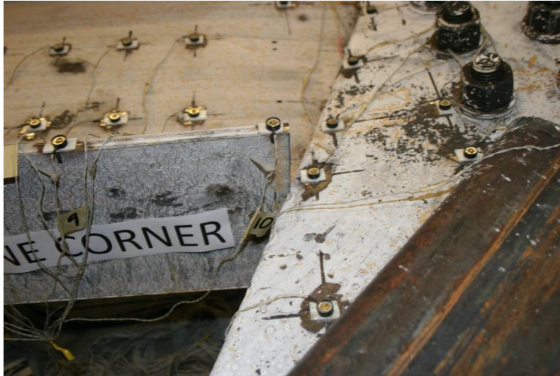
Figure 5-67: Contact Between Inner Beam Flange and Edge of Gusset Plate (2.7%)
