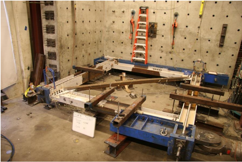
Figure 5-61: Initial Brace Global Buckling (PS B1, 0.4%)
