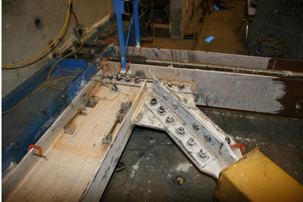
Figure 5-93: Damage in SW Corner End of Test (5.2%)
