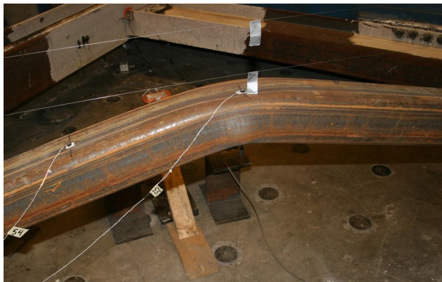
Figure 5-74: Brace Hinging Prior to Fracture (5.0%)
