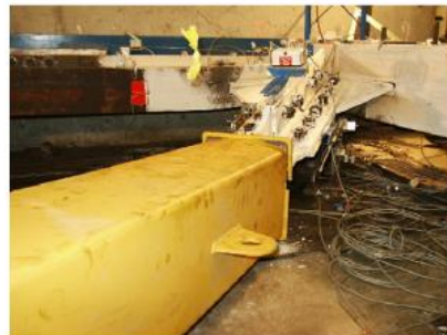
c) OOP Deformation Noted with All Specimens
