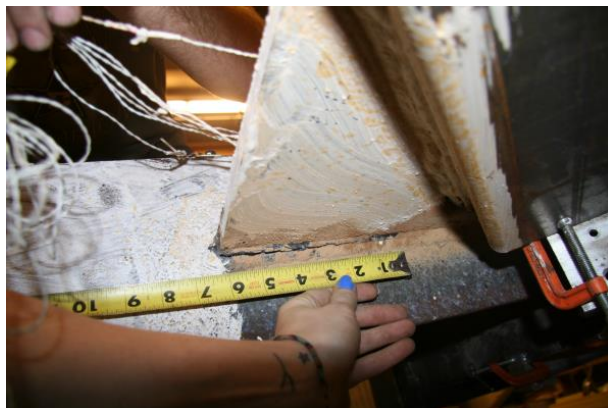
(2) Initial Weld Tear in Beam-to-Gusset Plate Weld
