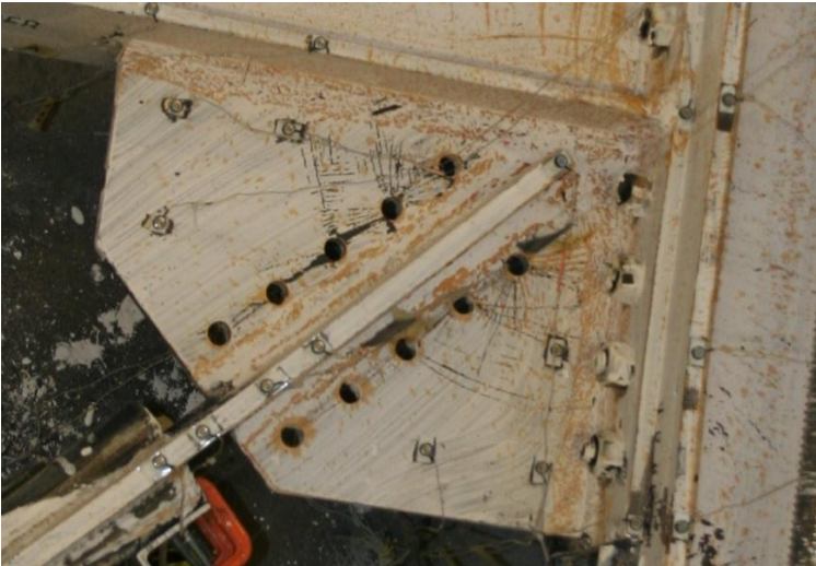
Figure 5-34: Moderate Yielding in NE Gusset Plate (PS Y2, 3.6%)
