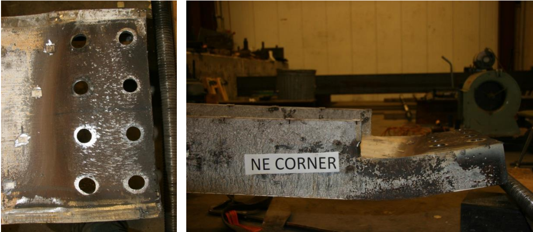
Figure 5-79: Damage to the NE Beam Web at End of Test (5.0%)
