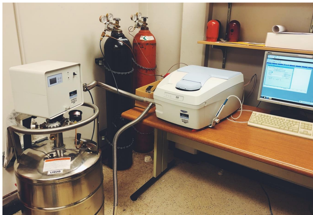
Figure 5.3. Perkin Elmer DSC 8500 used to determine the heat capacity of the sample solution.
