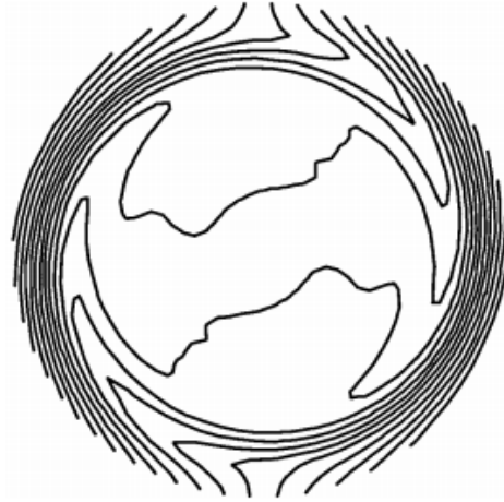
Figure 7.7: RMF field lines inferred from TCS experimental data. From ref [25]
