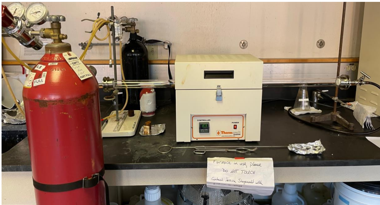
Figure 3.1 Thermcraft Tube Furnace with a sealed quartz process tube, nitrogen tank, flow meter, and influent and effluent tubing.
