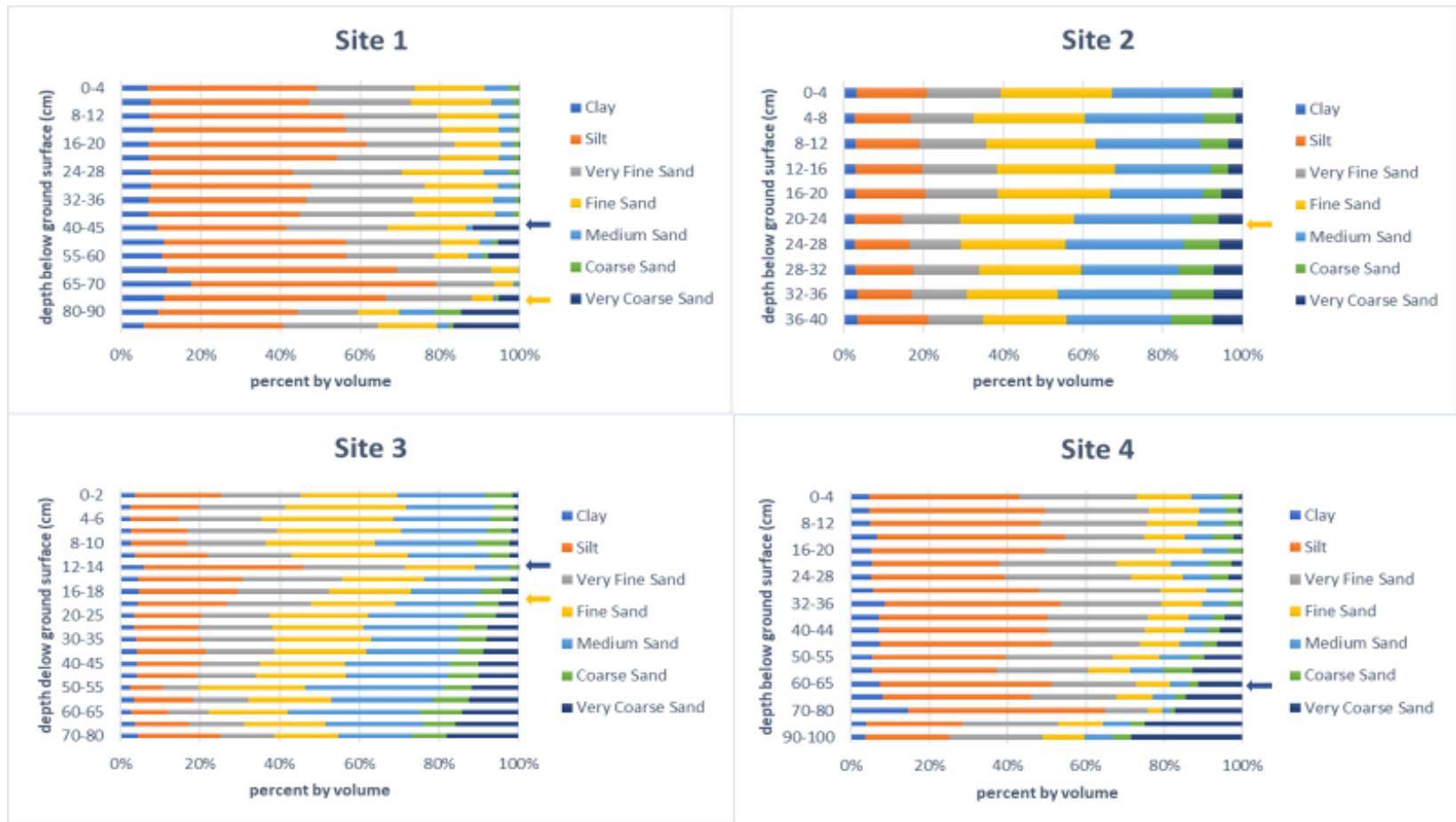
Figure 13 Grain-size distribution plots of the four coring locations. The approximate depth that corresponds to Interstate 5 construction is indicated by a blue arrow, located to the right of each plot. The approximate depth that corresponds to causeway construction is indicated by a yellow arrow. Samples collected at site 4 did not extend far enough beneath the surface to contain the causeway construction depth.
