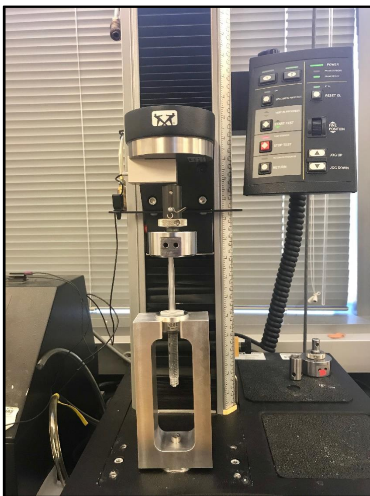
Figure 4.2. Custom-built syringe testing fixture for use with the INSTRON to measure the syringe glide force.
