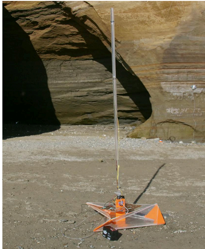
Figure 45 - Tensegrity antenna, digital model vs physical model
