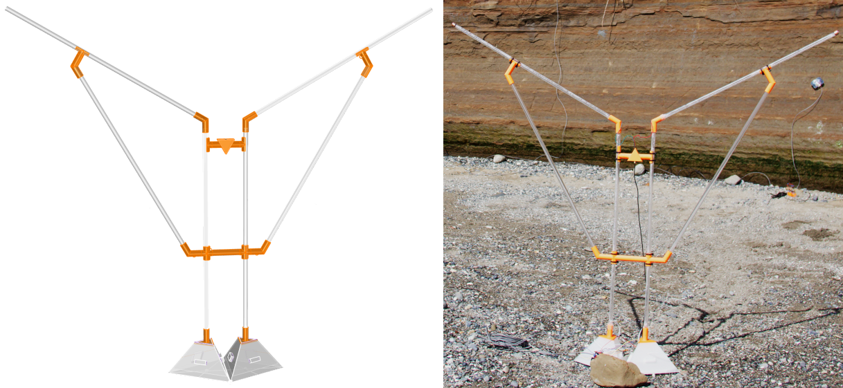
Figure 50 - Dipole antenna, digital model vs physical
