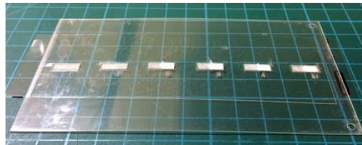
Figure 48: Construction protocol for 6x array of LFT-iSDA integrated cartridge devices: this format was used to increase test throughput and fabrication time.
