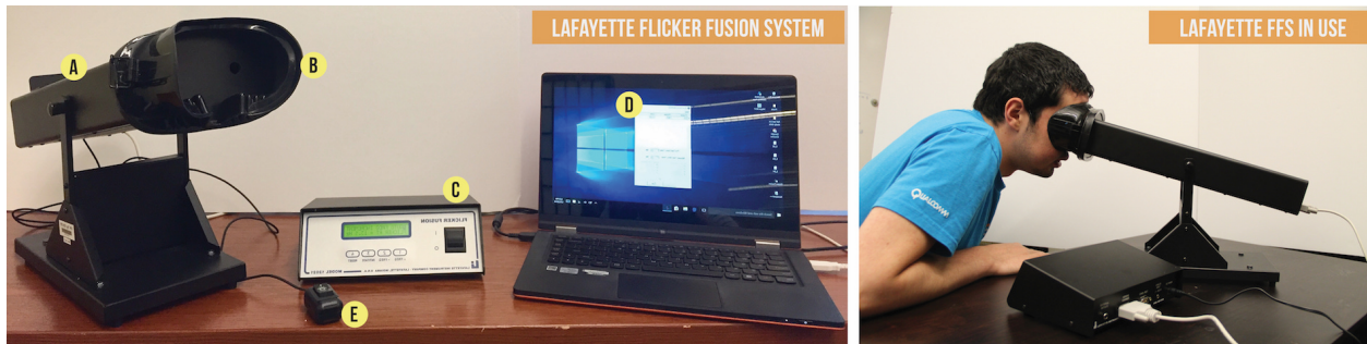
Figure 5.3: Left: The Lafayette Flicker Fusion System (Lafayette FFS) has three components: a viewing chamber with the light stimulus (A, B), a controller (C), and a software program to record results (D). The clicker (E) is connected to the viewing chamber and records a person's input (i.e., indicating they see a flickering light or a fused light). Right: To use the Lafayette Flicker Fusion System, a person presses their face against the mask covering the viewing chamber so as not to allow any outside light. The person then focuses on the light inside the viewing chamber and uses the clicker to record their input.
