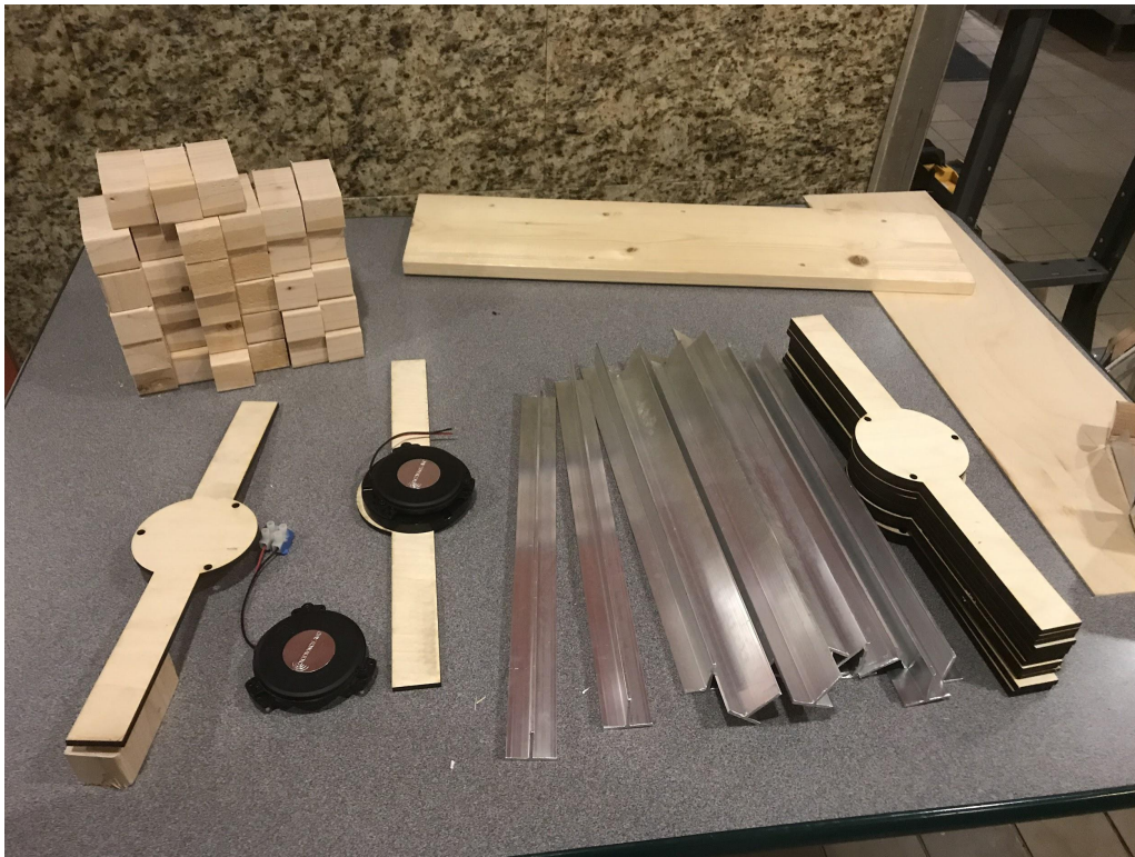
Figure 46 - 17' driver bridge segments before construction
