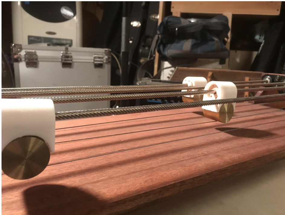
Figure 3 - "AutoSlide Instrument", view of brass slides and carriages along leadscrew, 2018
