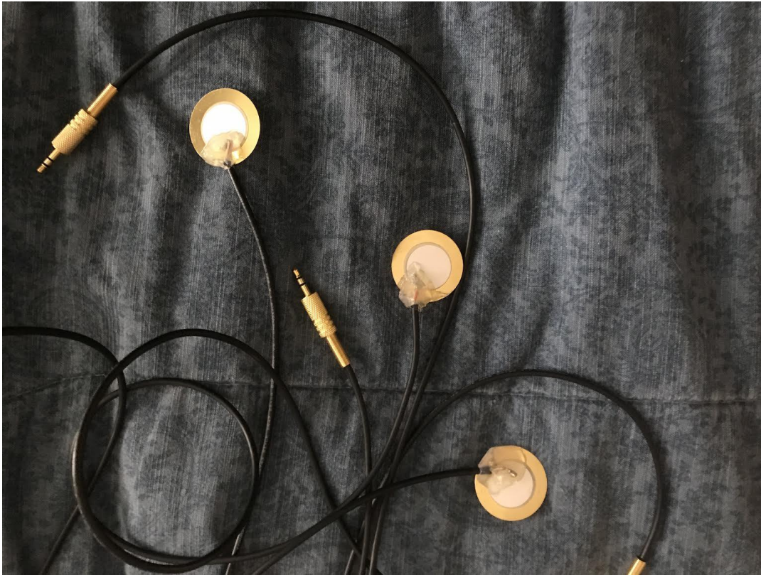
Figure 38 - Hand made contact mic with piezo elements
