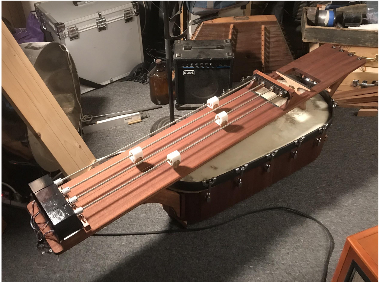
Figure 2 - "AutoSlide Instrument", view of top with leadscrew and motor housing, 2018
