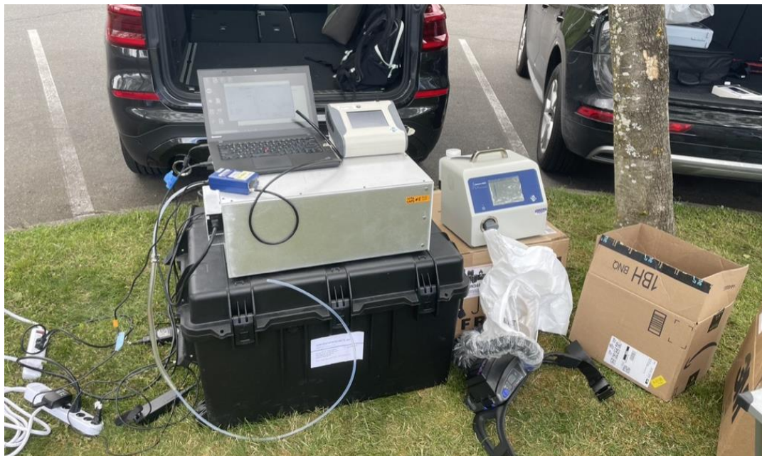
Figure 4. Direct reading measurement instruments set up for measuring environmental exposures at the site.
