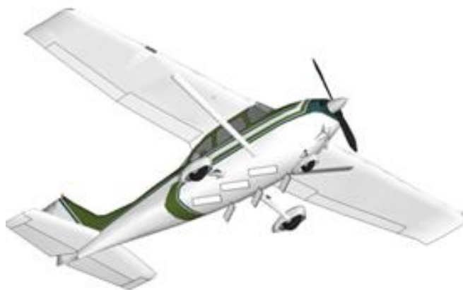
Figure 2.4. Forward- and aft-squinted antennas on the starboard and port side of the aircraft
