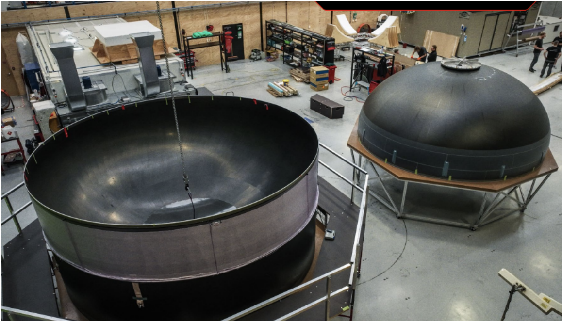
Figure 1.2: Composite-based rocket fuel tank made by Rocket Lab [3]. This particular one is made in two parts, whereas this project will be making a tank out of one continuous part.
