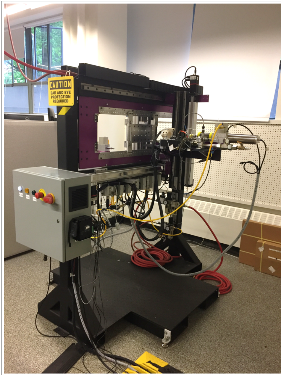
Figure 2.1: Displays the black steel box tube frame with large footprint used to support the test bench, showing mainly the right-hand side. The valve manifold is located beneath the (purple) coupon holder, and two pressure filtration-lubrication regulators are attached to the far lower side of the steel frame.
