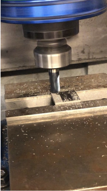
Figure 8: Haas CNC mill: spindle shown cutting a CT specimen
