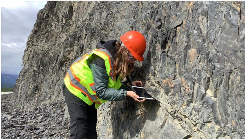
Figure 2.1 Measuring orientation of a fault at Long Lake 71 using the Geopad system.
