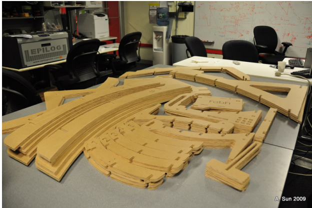
54. Laser cut pieces pre-assembly for Fabfi reflector
