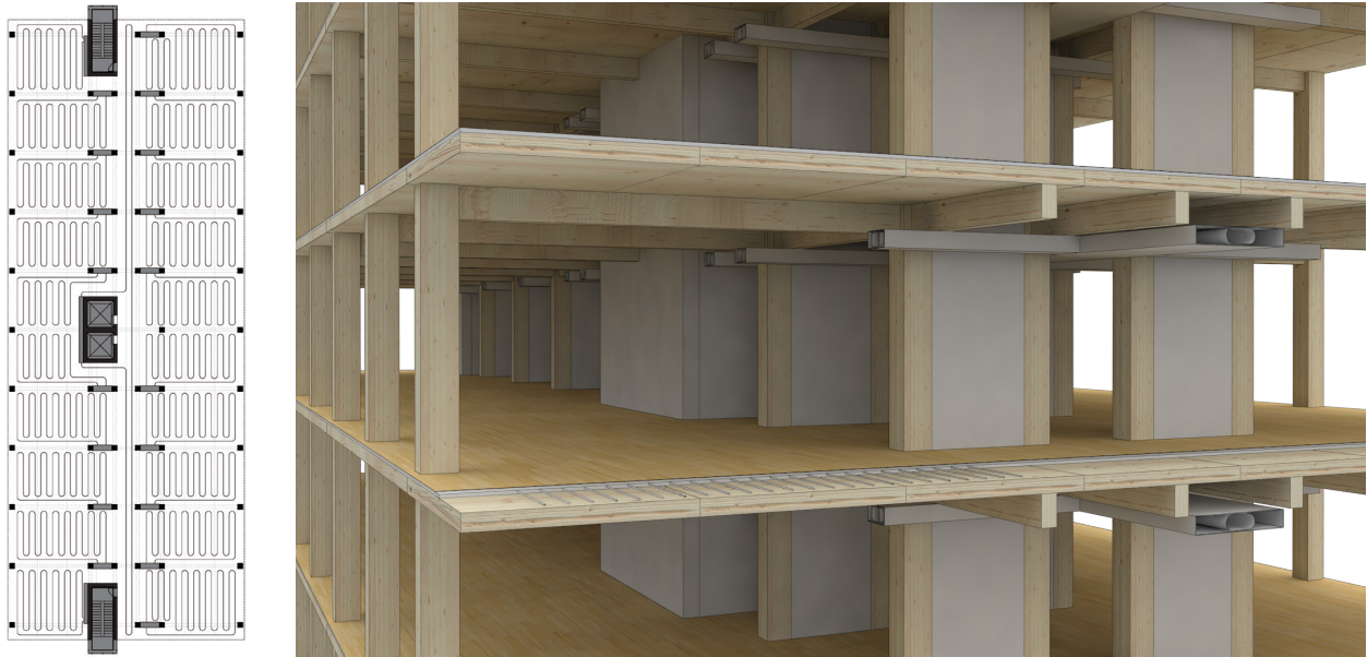
Fig. 8-7 Horizontal Distribution & Dedicated Systems. The example shows a radiant in-floor system providing thermal heating and cooling while operable windows and a under structure, low profile, duct system maintain a healthy air exchange. Electrical distribution follows the main vertical chases and additional partition walls or be distributed horizontally under the drop ceilings or conduit systems depending on aesthetic and/or programing choices of the user.
