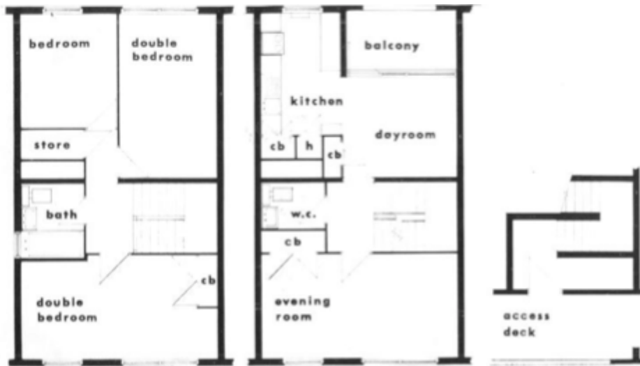
Floor plan for a 5 person deck access house in the Towers. Deck Housing at Killingworth . Newcastle Libraries.
