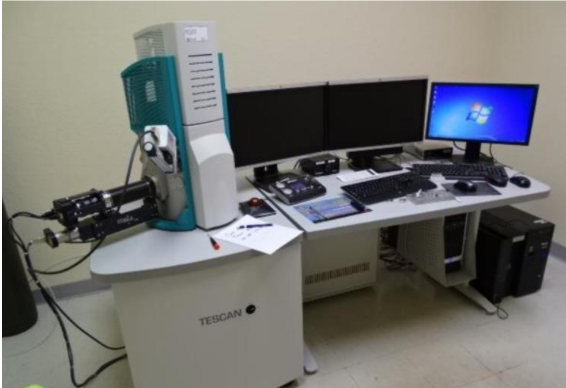
Figure 2-7. The TESCAN VEGA3 XYZ scanning electron microscope/electron beam lithography machine
