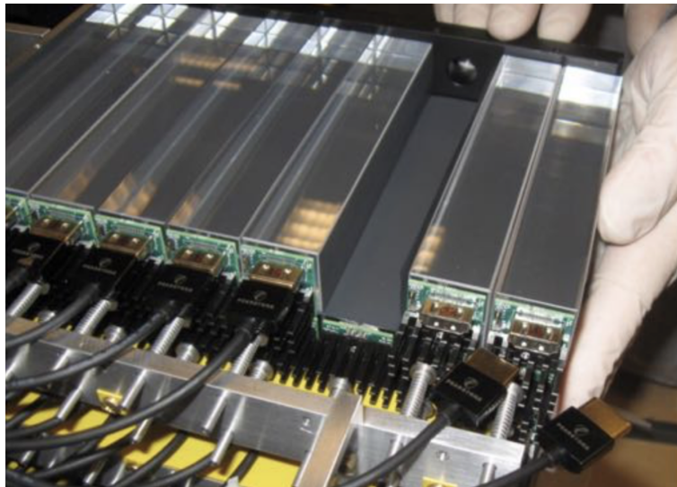
Figure 2.9 – Each calorimeter consists of a 9x6 array of PbF 2 crystals with attached silicon photomultiplier (SiPM) chips. The SiPMs detect the Cerenkov light produced in the crystals when a positron passes through a calorimeter. Image credit: [48]
