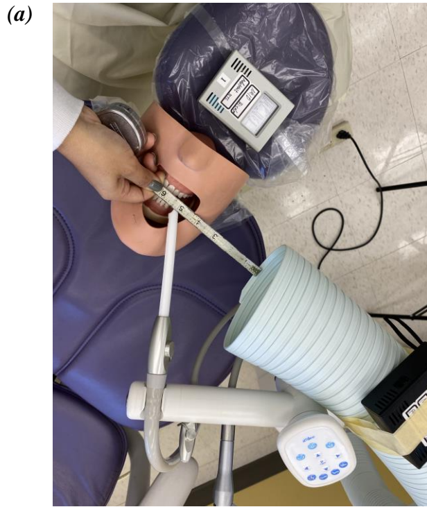
Fig 4. Images of typodont setup with manikin cheeks in place, attached to the head of the test chair. (a) The opening of the EOS was positioned 6" away from the typodont central incisors, on the left side of the chair. (b) The IOS was placed 1" above or below the incisors during the attachment removal of the lower and upper arches, respectively.
