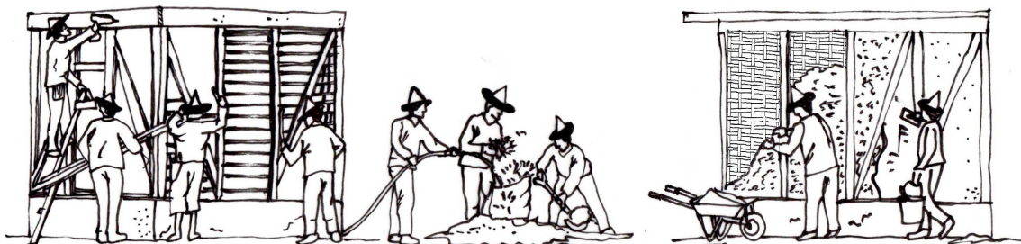
Image: Wattle + Daub construction (similar methodology to CFB)
