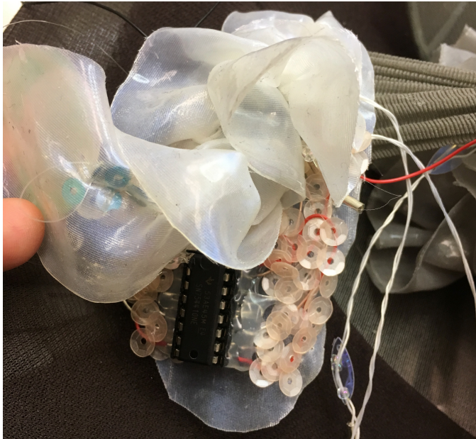
Figure 2.1.3-17 Embroidered circuit with DC motors (Attiny85 + H bridge). Photography by the author.
