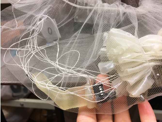
Figure 2.1.3-14 Circuit with vibration motors (Attiny85 only). Photography by the author.
