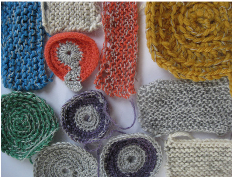
Figure 3.3.1-1 Crochet pressure sensors (Kobakant) 16.
