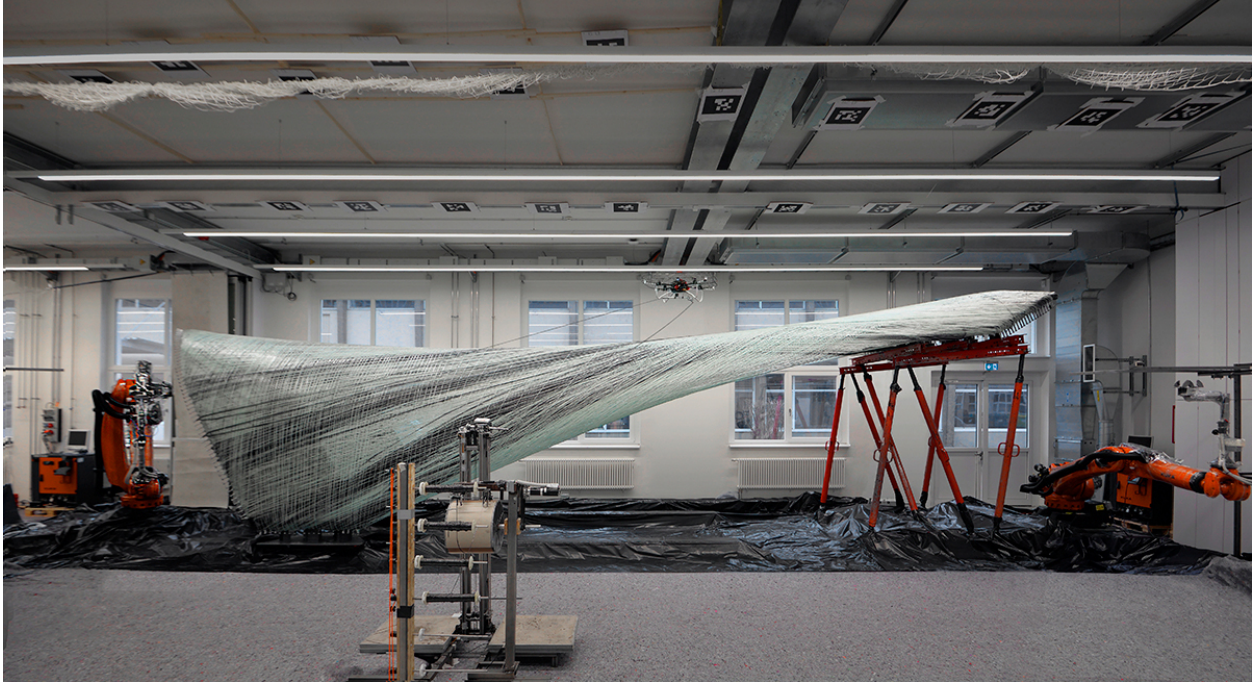
Figure 6 Robotic fabrication of the pavilion (Felbrich, et al. 2017)
