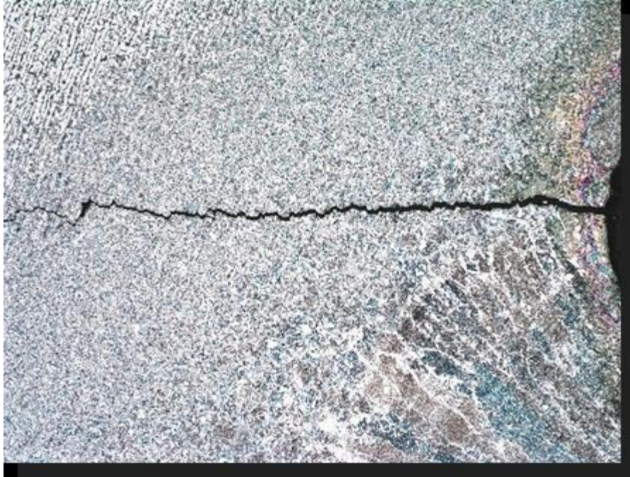
Figure 6.13 Un-Peened Test Sample 4 Crack Site
