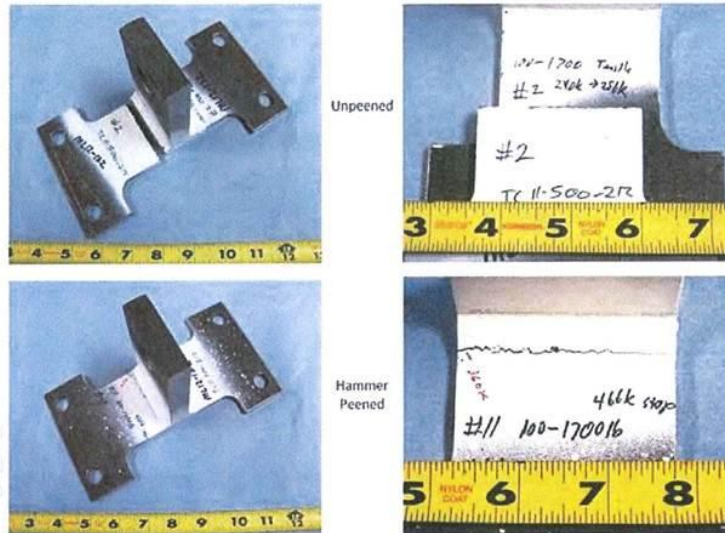
Figure1 — The reference unpeened fillet welds shown at the top fractured in 256,000 cycles, while the hammer peened welds at the bottom were cycled to 466,000 before cracking.
