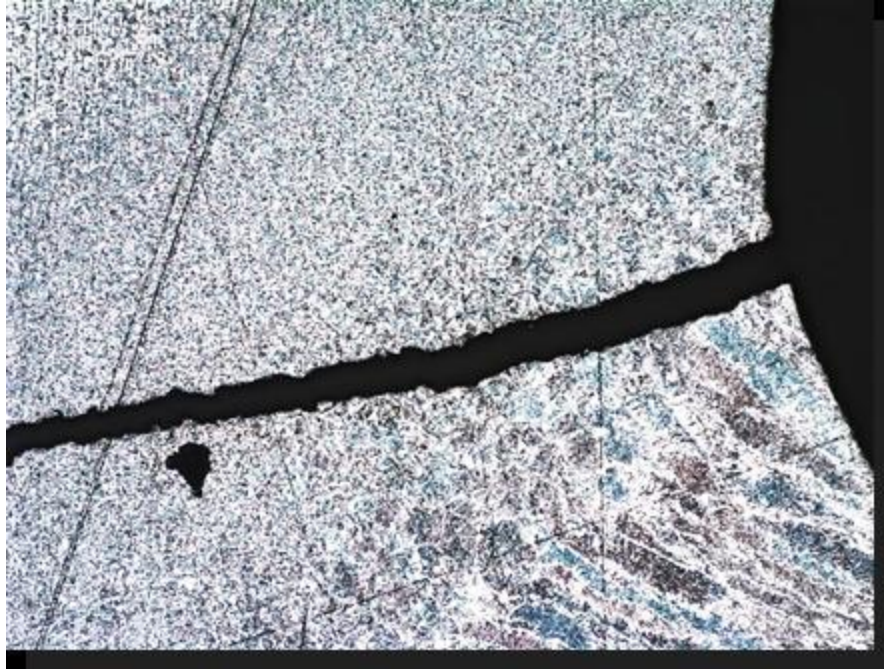
Figure 6.15 Flap Peened Sample 22 Crack Site
