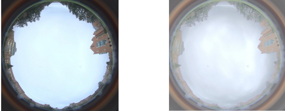
Figure 5 Reinhard photographic tone-mapped image of a Radiance HDR file of the sky (left) and Ward's Histogram based Tone-map of the same HDR Image (right)
