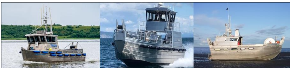
Figure 14: On the left is a “stern-picker” style drift gillnet vessel. In the middle shows a thru-picker. On the right shows a bow-picker style vessel. (Left-to-right: Photo 1: Jim Purdum. Photo 2: FiskerForum.com. Photo 3: permitmaster.com).
