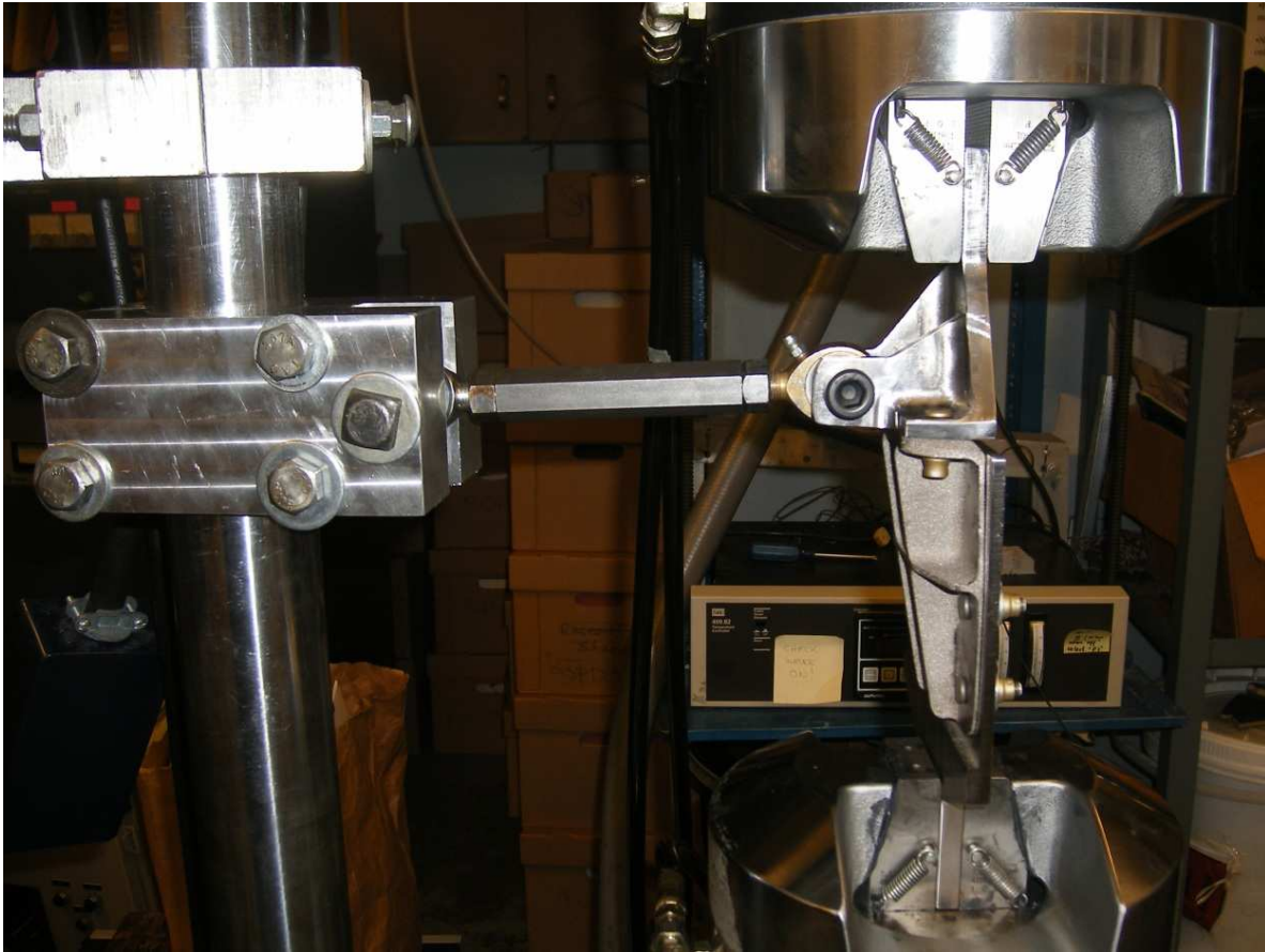
Figure 6-27: Cyclic loading test setup with the rigid link on the load frame and fixture
