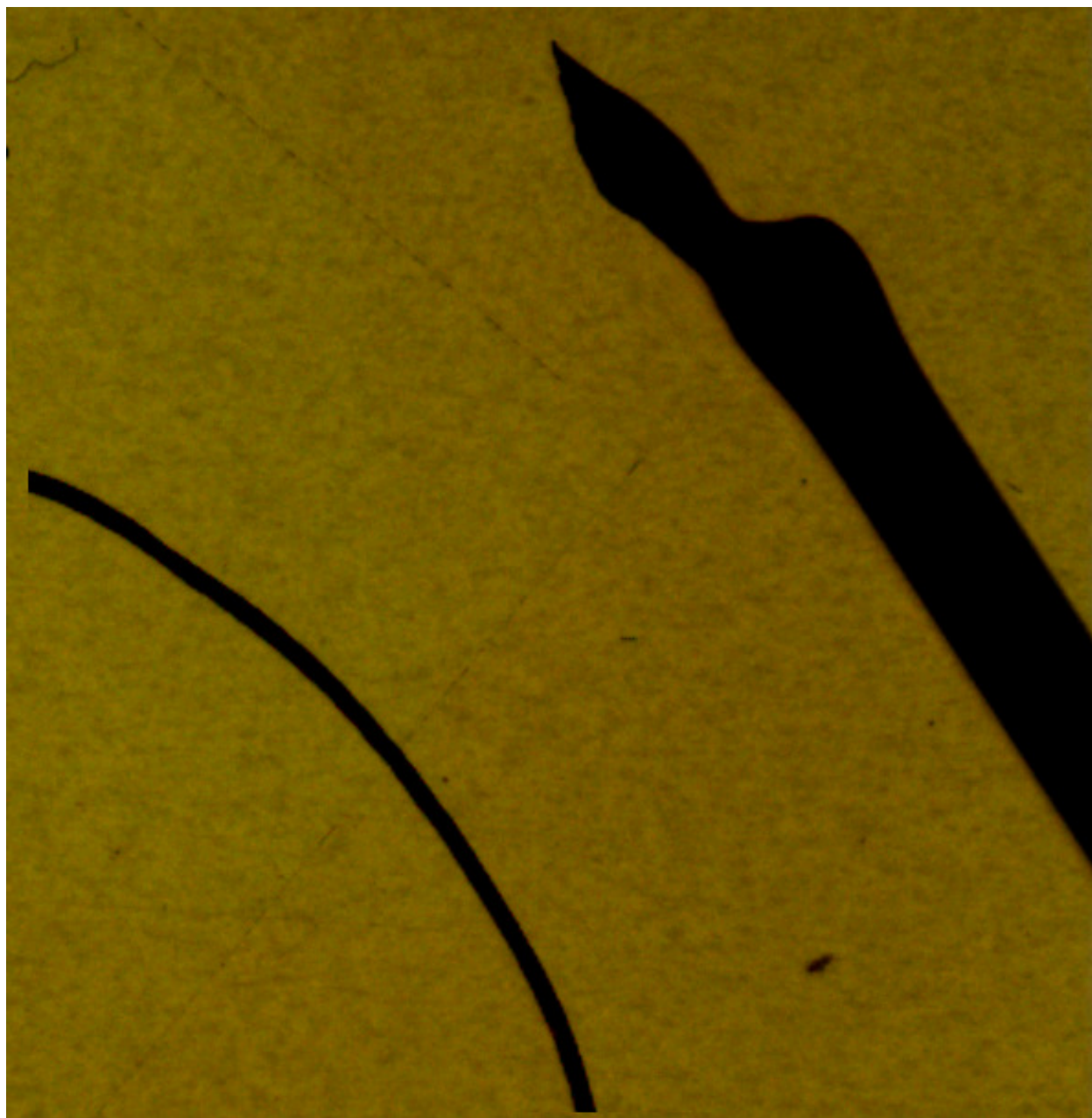
Figure 82: pH-dye observations around mechanical sensor components. No pH-dye color change, or pH-dye color gradients are seen next to the ribbon (left) itself, or the beam holder (right).
