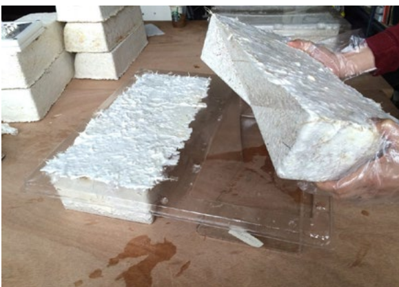
Figure 24: Hy-Fi Project brick molds
