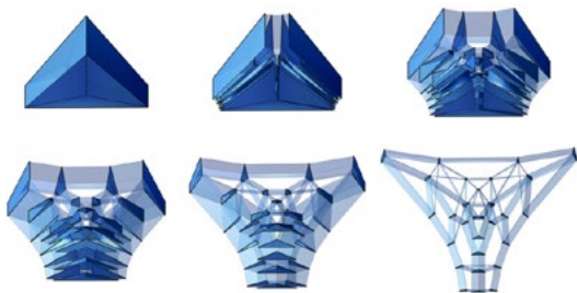
Figure 27: MycoTree polyhedral structural form diagram
