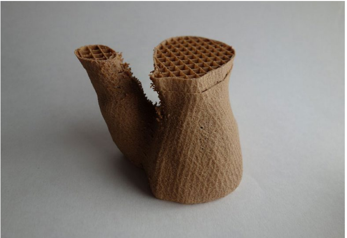
Figure 37: 3-D printed segment of straw core.
