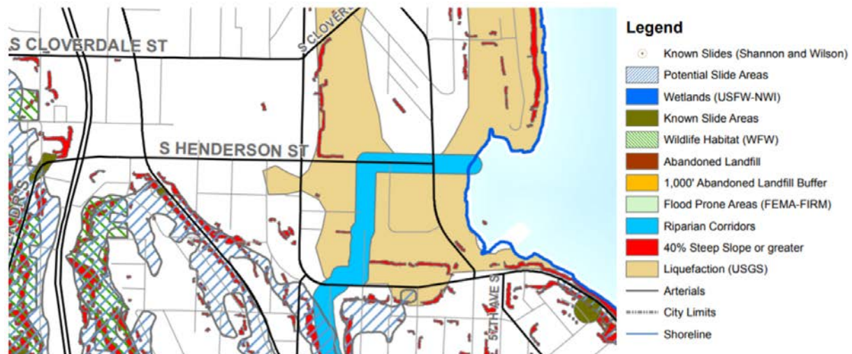
Figure 75: The stretch of S Henderson Street that is east of Rainier Ave S is in a moderate to high liquefaction zone. (Source: City of Seattle Department of Construction and Inspections).
