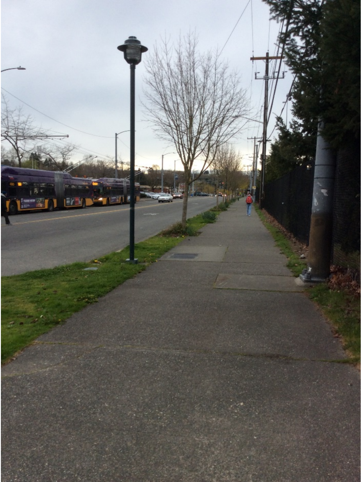
Figure 6: This stretch of pedestrian ROW is on the north side of S Henderson Street, between 52nd Ave S and Rainier Ave S. The sidewalk is 10-feet wide and is accompanied by a planting strip. (Source: Kaylie Duffy).
