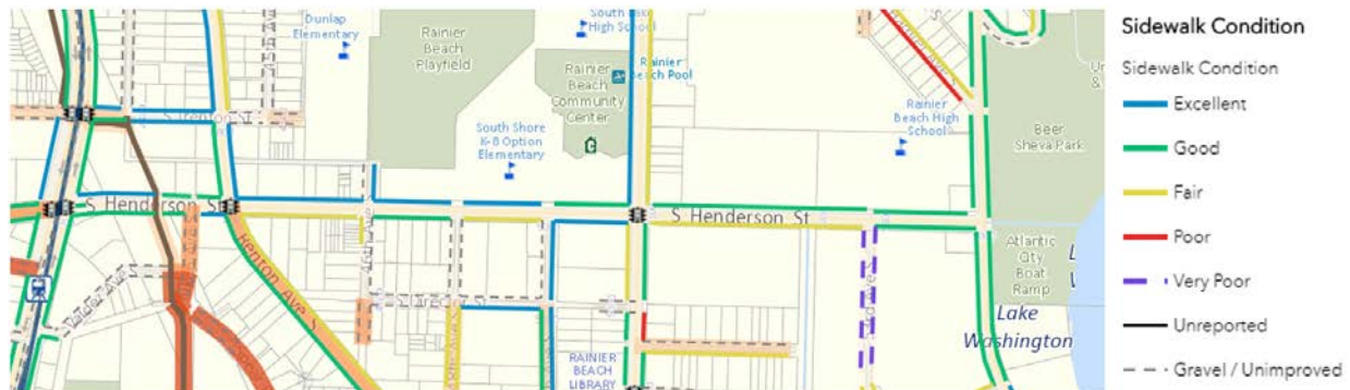
Figure 18: SDOT's evaluation of S Henderson Street's sidewalk conditions. (Source: SDOT).
