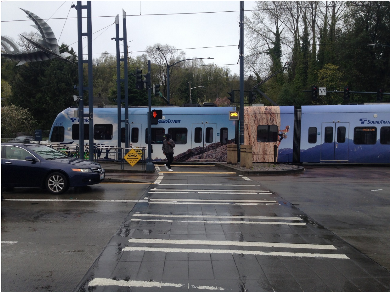
Figure 70: A southbound Sound Transit light rail vehicle arrives at the Rainier Beach Station. Note the lack of crossing gates on the station platform. (Source: Kaylie Duffy).
