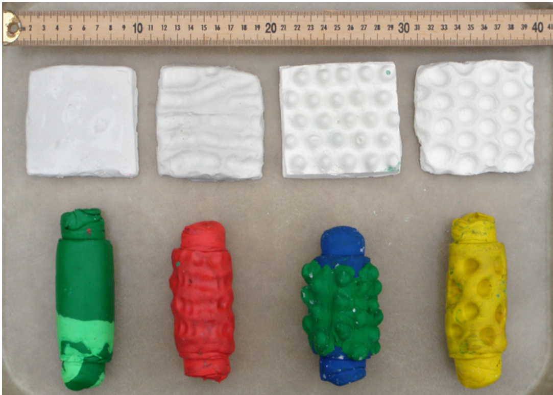
Figure 1: Plaster molds of tiles and clay cylinders. From left to right: flat(unadorned), furrowed, raised bumps, inset wells.
