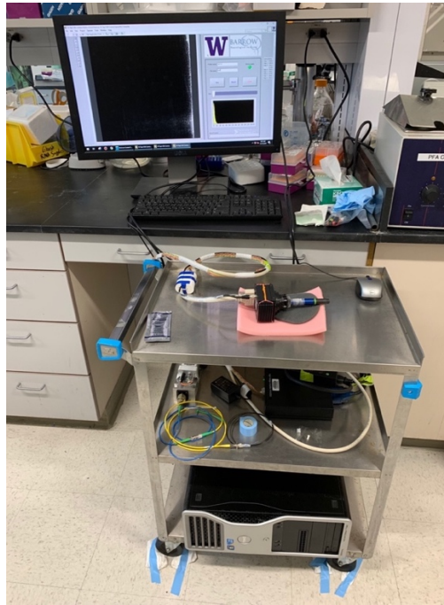
Figure 5.1 The handheld LS-DAC system set up in a standard surgical cart at the BNI. The system can safely transport between the operation room for imaging and a safe location for storage.
