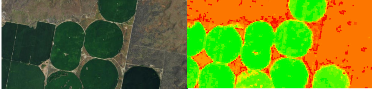
Figure 2.2 (a) Pre NDVI processing (b) Post NDVI processing (GIS Geography, 2018)
