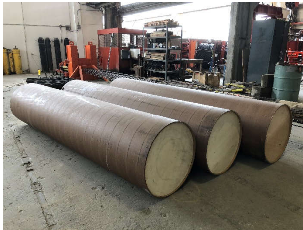
Figure 7-9. Sonovoid® Round concrete void forms
