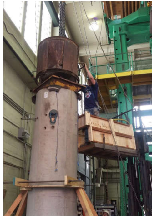
Figure 7-20. Casting plug inside of column
