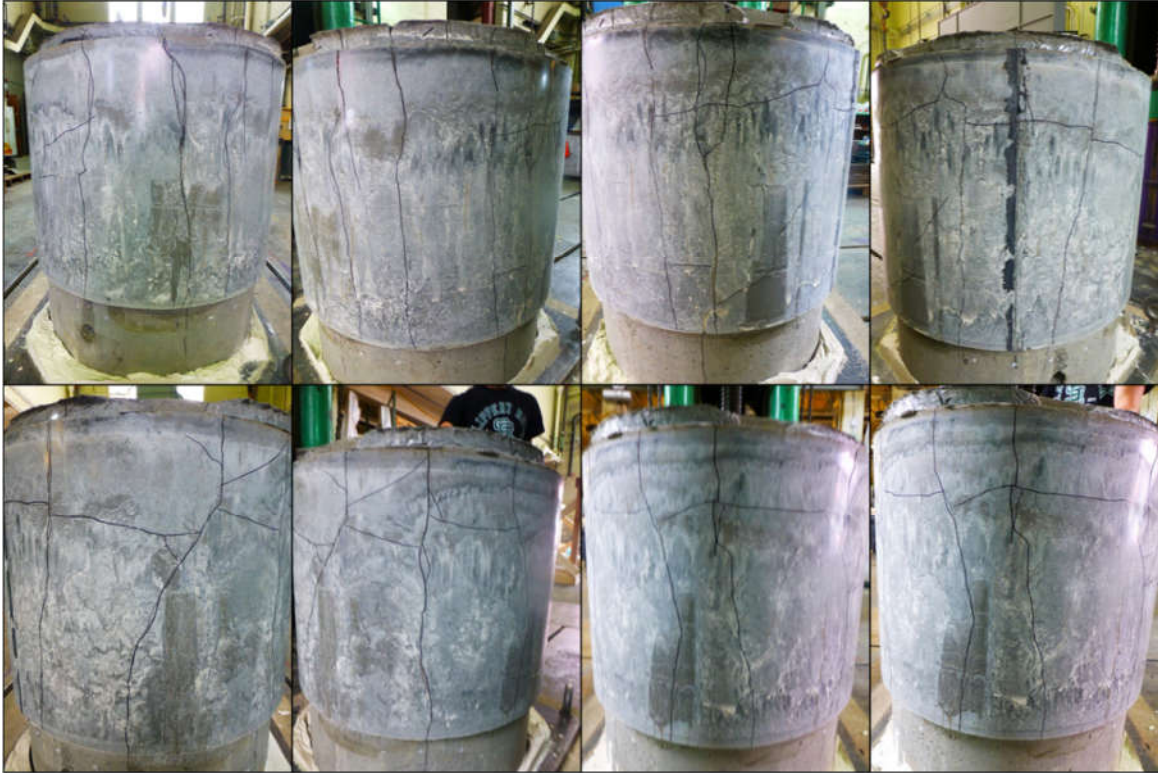
Figure 5-17. Crack Formation at end of testing for Test ep24s1-1 (L-R: N-NW-W-SW; S-SE-E-NE)
