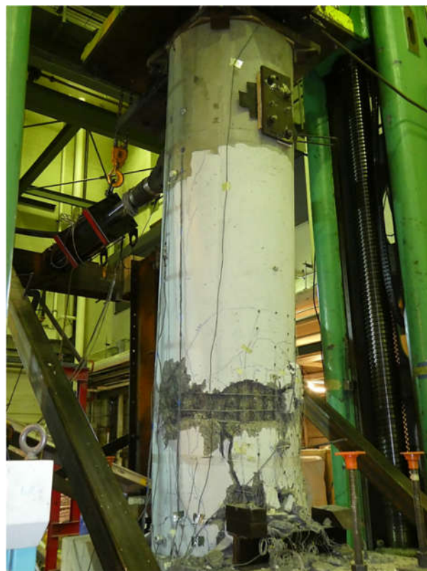
Figure 8-16. Final position of specimen at failure
