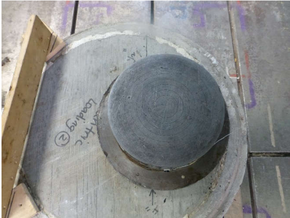
Figure 4-7. Load Bearing Plate shifted off-center for Eccentric Load Test
