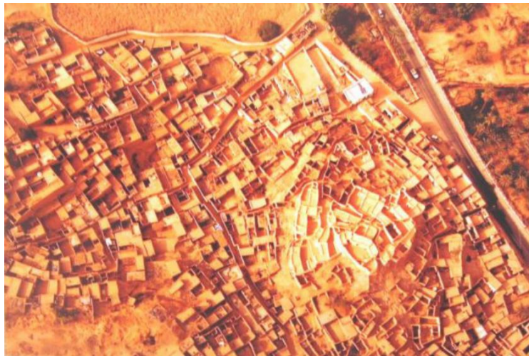
Figure 20 - Mass plan of Ksar El Mihane in Djanet as a typical compact cellular layout
