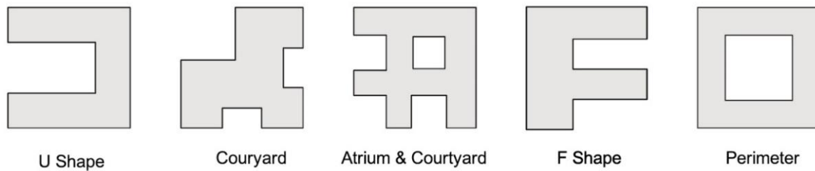
Figure 38- The footprint of the generic geometries at ground level -Typologies inspired from a previous study [46] for lot coverage
