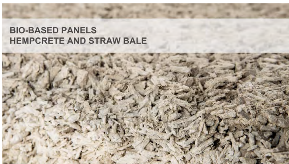
Figure 20. Hempcrete insulation derived from hemp shiv and a lime-based binder.
