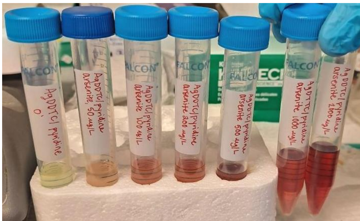
Figure 78. Arsenite color development in AgDTC/pyridine. Noticeably improved color distinction from 0-2000 ug/L As.
