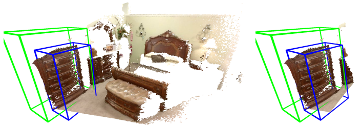
(a) An example of predicted bounding-box with the whole pointcloud. (b) An example of predicted bounding-box from the cropped pointcloud.
