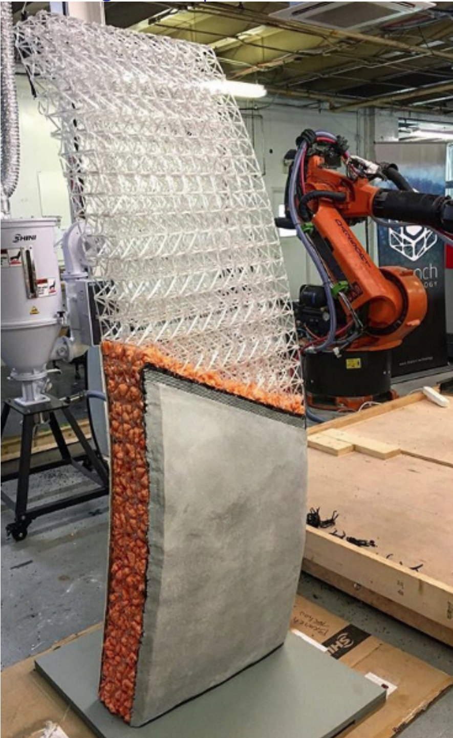
Fig. 128: A Demonstrative Curved Wall Panel by Branch Tech. Branch Technology https://www.branch.technology/process
