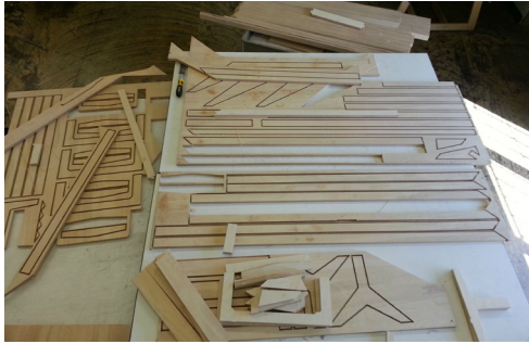
Fig. 13 CNC cut plywood
