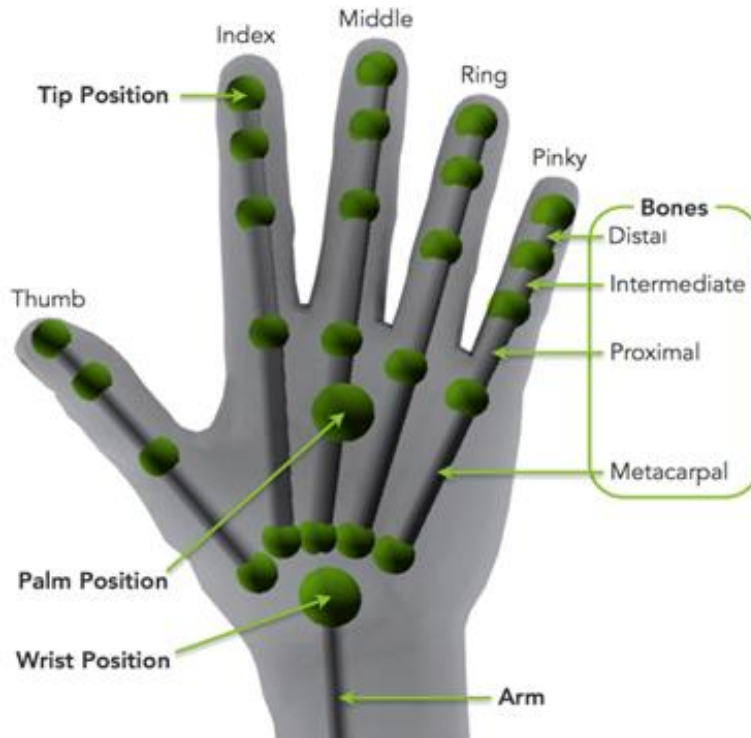
Figure 4.3.2. Example kinematic output from Leap Sensor API [38]. The Leap sensor provides direct access to individual joint positions (green spheres) as well as direction vectors (grey bars) of up to two hands at a time.
