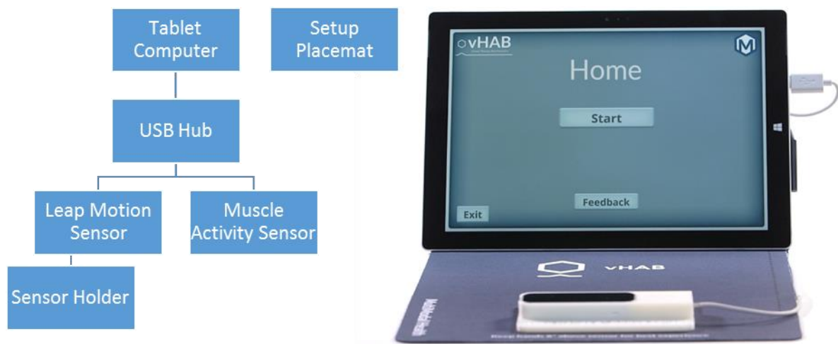
Figure 4.3.1. Block diagram of vHAB hardware components and image of assembled Home system. Individual hardware pieces are connected through a combination of wired and wireless methods while accessories aid in system setup and use.
