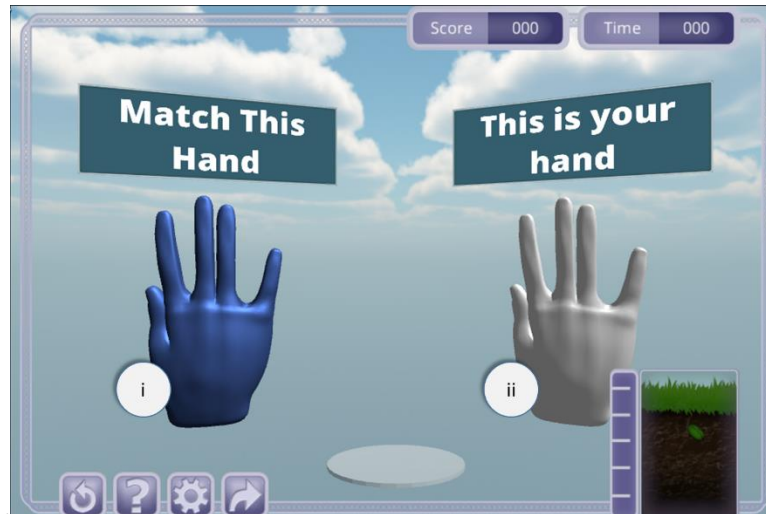
Figure 4.4.26. Finger Position Match Game. In this game, patients must adjust the positions of their fingers to control a virtual hand (ii) and match a target hand (i). Finger positions are represented in a set of finger touch states that indicate whether or not two fingers are touching each other. The above state is 1) true, 2) false, 3) true, 4) false.
