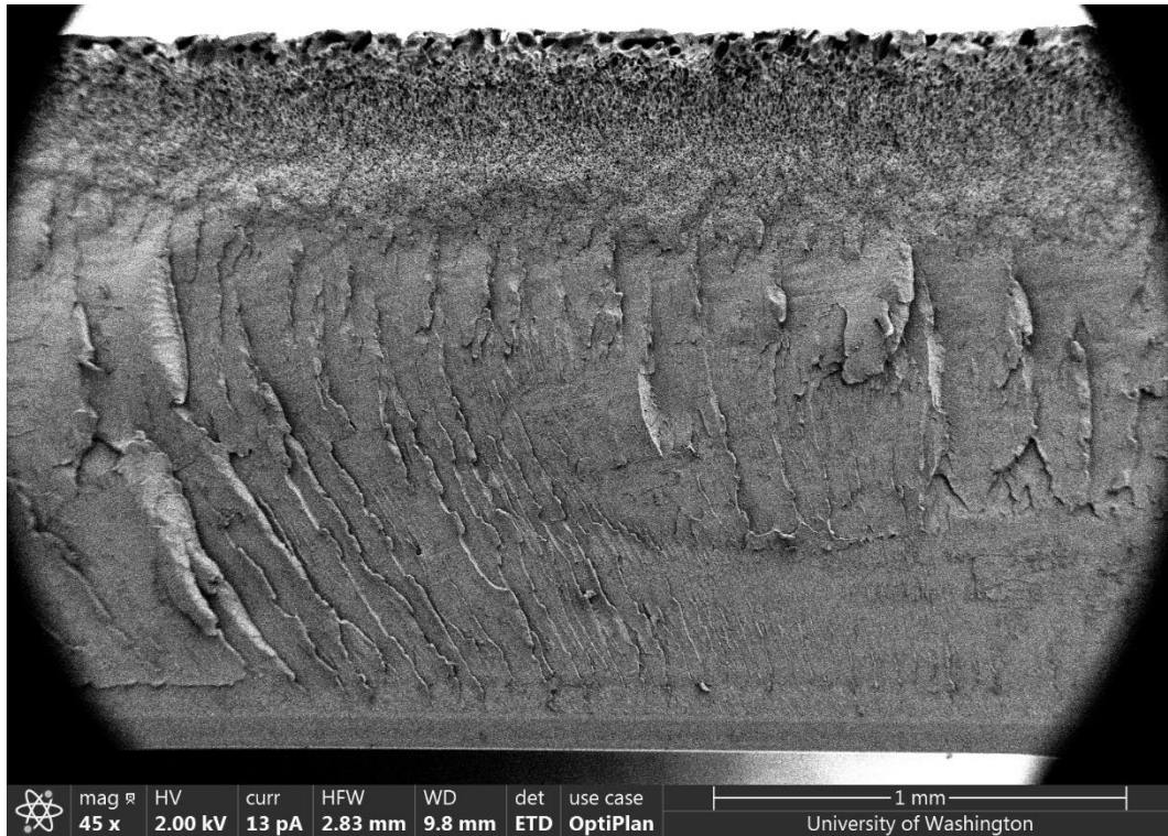
Figure A.24a: Full thickness micrograph. The foamed side is at the top of the image.
