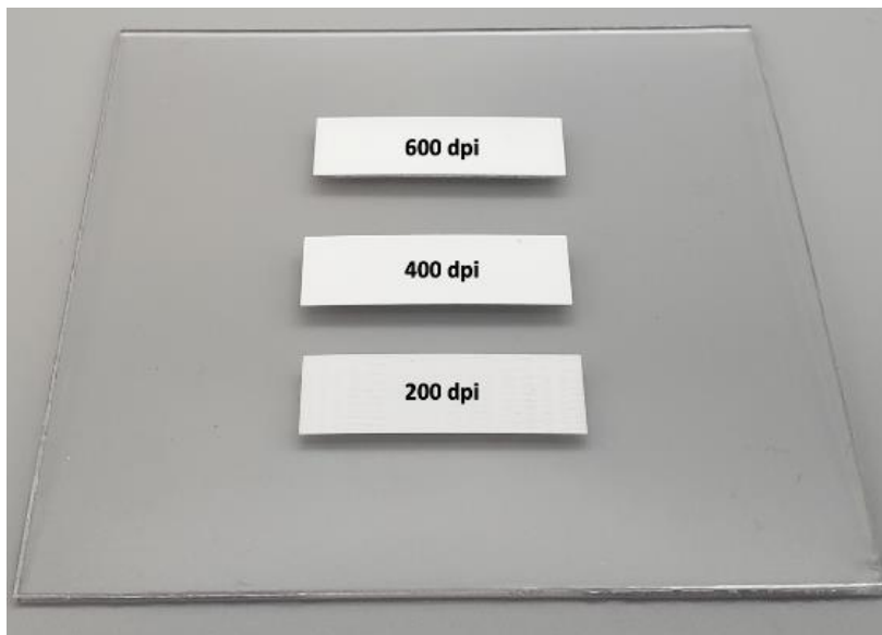
Figure 16: Different DPI settings foamed on one specimen
