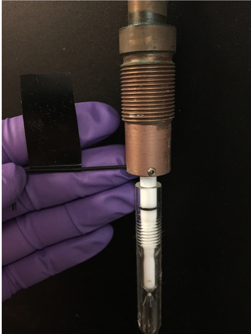
Figure 4-10. Tightening one of two set screws to secure Teflon pin. By tightening the set screws, the Teflon cap will not be loosened while manipulating sample during pressurization.
