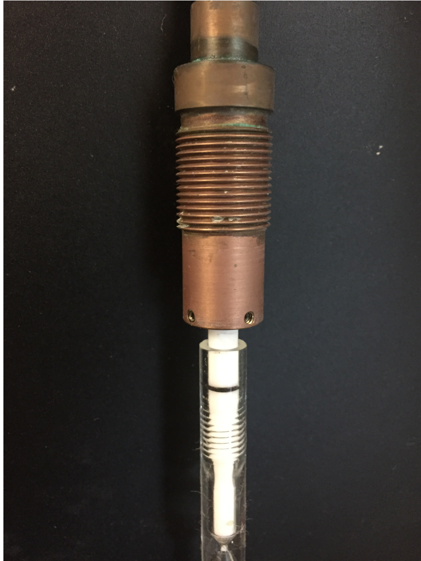
Figure 4-11. Both set screws tightened. The sample is ready for the plastic protective sleeve.
