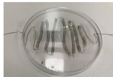
Figure 2: Shaped nichrome wire taped in place with petri dish placed on top to show its size
