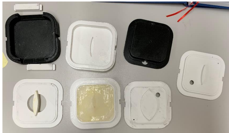
Figure 1: 3D printed molds used for making the model
